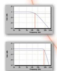
The Filter board in combination with the AFL-6400 system is using such a filter for each input and output, in order to provide a higher bandwidth (80 Khz. instead of 50 Khz. for our example) while reducing the input noise and providing a smoother output signal (with less noise and less "stairs" at an excellent Signal to Noise ratio.
