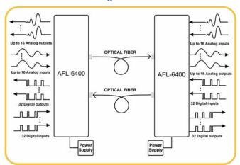
The product is based on A/D and D/A technique, combined with a powerful transceiver, for ranges of up to 100 Km, at analog bandwidth of up to 250 KHz. per channel, at 16 bit resolution (96 dB S/N ratio)
